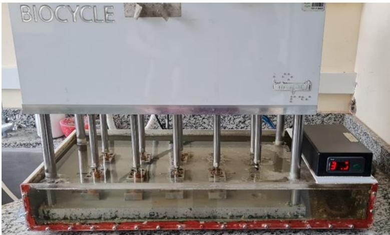
Figure 4: Samples accommodated in the pneumatic cycler.
